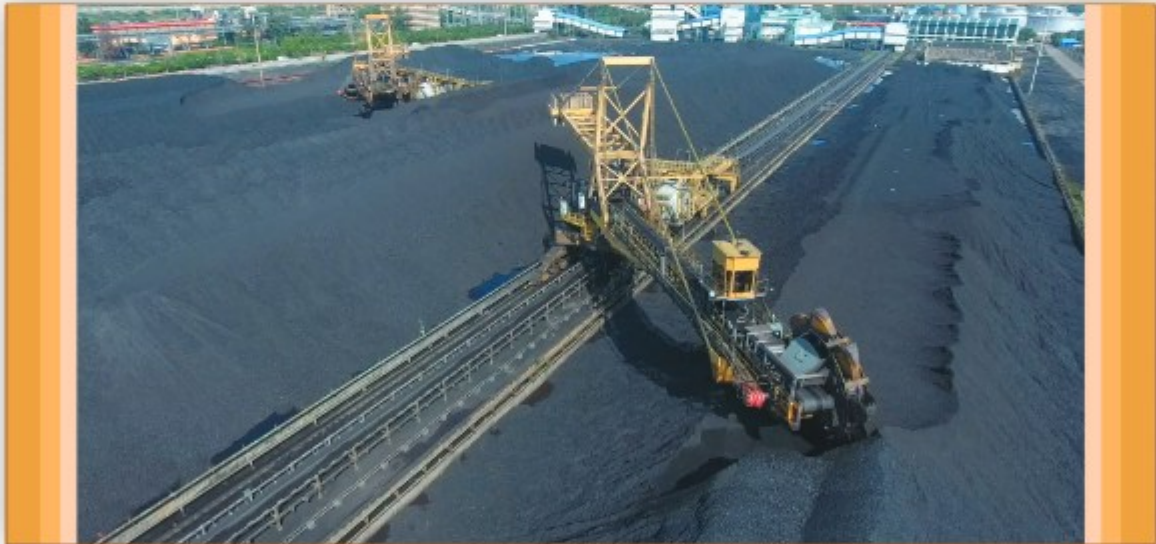
Coal Stock Yard
